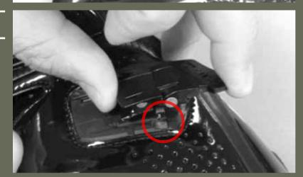
PRESS NEW BUCKLE DOWN TO ENSURE TAB GOES INTO RECEIVER
